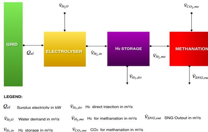
Figure 3: Concept of PtG modelling used in the study
